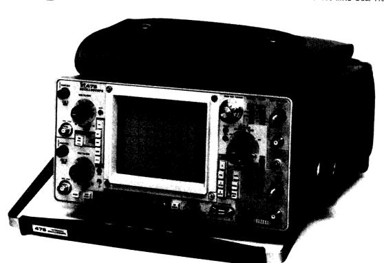
475 pictured above is identical in appearance to the 465 (not shown) except the 465 deletes the 0.01 and 0.02  $\mu$ s TIME/DIV and 2 mV VOLTS/DIV switch positions.
